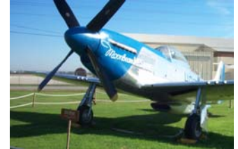
P-51 Mustang on static display at Barksdale AFB, LA Notice the yellow tips on each propeller blade. Even the big guys paint the tips to mark them as a safety hazard. (Photo by Jim Orsborn)
