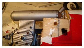
The next photo is the installed muffler and engine before the cowl is mounted. This last photo shows the cowl installed over the engine with the muffler cutout.
