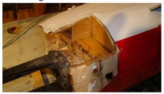
The first step in adapting the muffler was to make a cutout in the fuselage. The size and orientation of the motor were not suitable for a complete internal muffler installation, alterations on the cowl were necessary as will be
