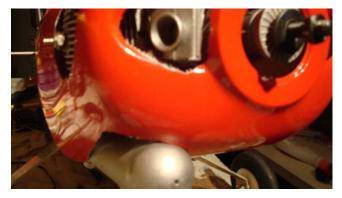
The exhaust comes out of the bottom of the fuselage which makes for a neat installation in this case.
