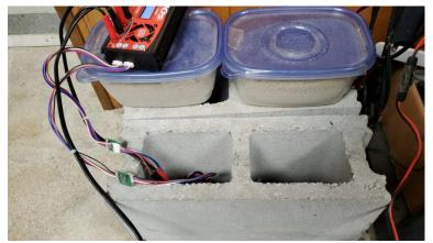
"I put the cells inside cinderblock on top of a paving stone. I put a plastic bin full of sand on top, the idea being that fire would cause the sand to dump into the cinderblock. The cinderblock also keeps groups of packs separate to limit chain reactions."
